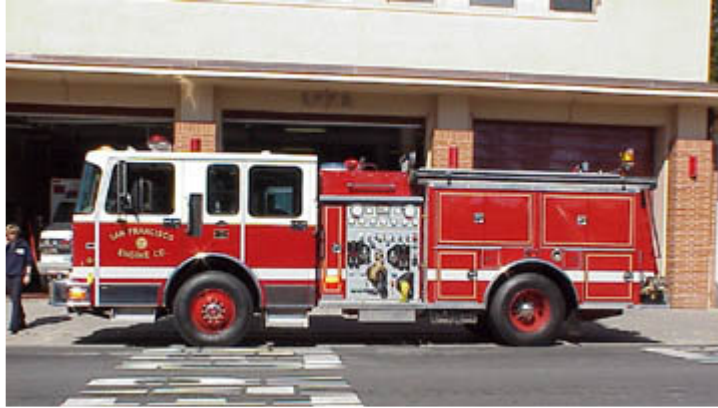
San Francisco Fire Department 1,500-GPM, two-stage pump
