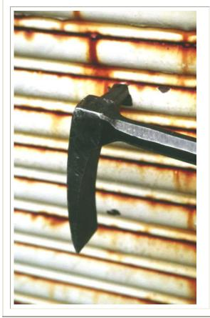
**Left and Below:** With slats that are difficult to remove, drive the point of the Halligan into the slat then drive the Halligan with a flat head axe or sledge.
