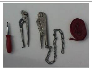
Above: Handy tools for forcible entry situations. From left to right, screwdriver, water-pump pliers (Channel Lock) with ends ground and bent to create "key" tools, Vise Grips for securing padlocks during cutting operations and pulling slats on roll-up doors, and webbing to control doors while they are being forced. These are just a few of the many uses.
